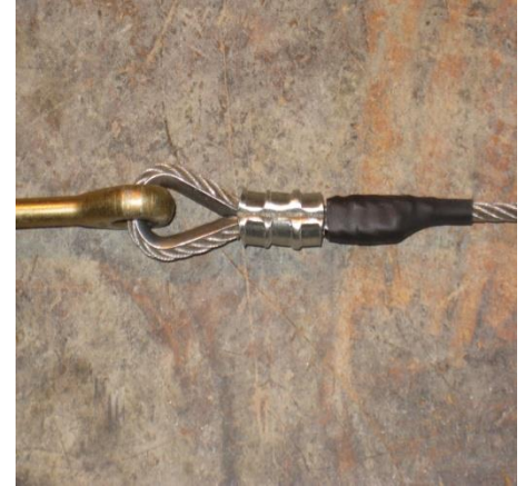
Figure 17 - Finished Cable End
