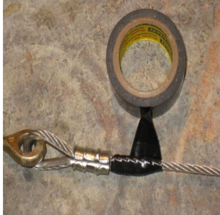
Figure 16 - Chafe Tape Installation
