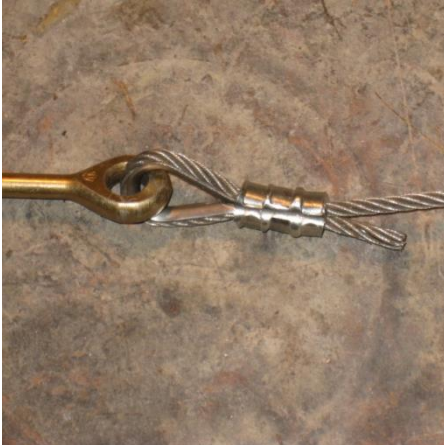
Figure 15 - Cable Finished to Length
