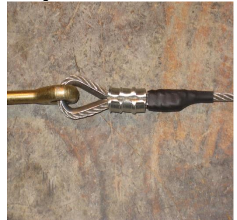
Figure 19 - Finished Cable End
