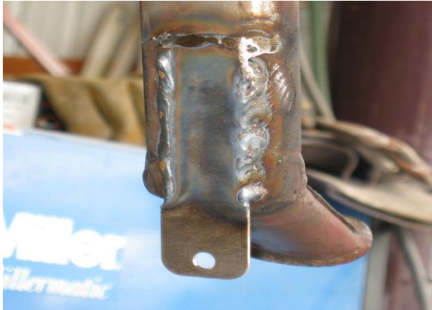
Figure 6 – Single-hole tang welded to step
