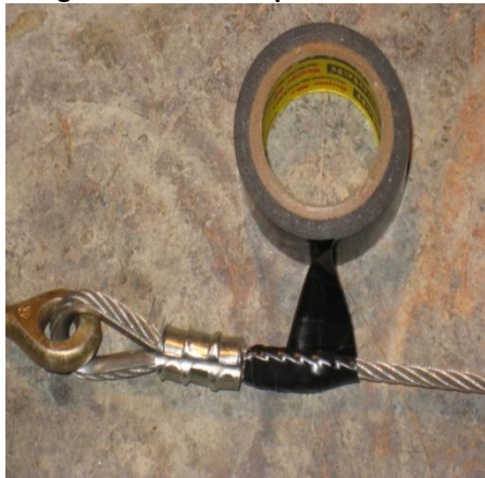
Figure 18 - Chafe Tape Installation
