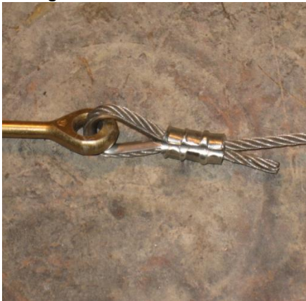
Figure 17 – Finished Cable End
