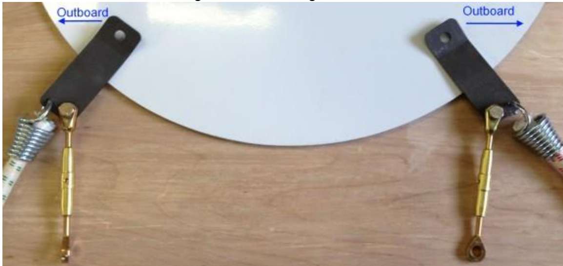
Figure 2 – Forward Tang Installation
