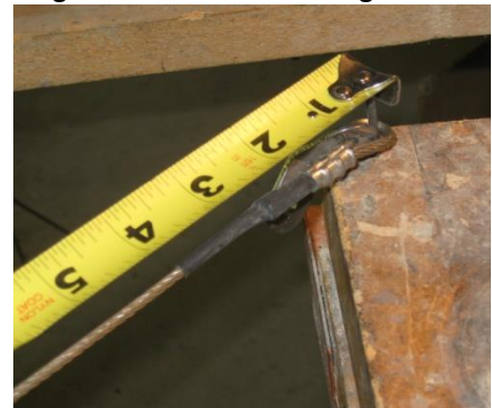
Figure 14 - Cable Measuring Fixture
