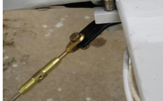
Figure 5 - Rear Limit Cable Installation
