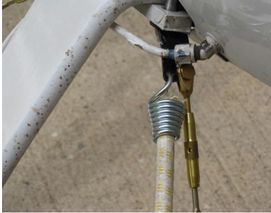
Figure 4 - Ski Front Cable Installation
