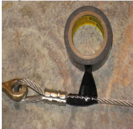
Figure 16 - Chafe Tape Installation
