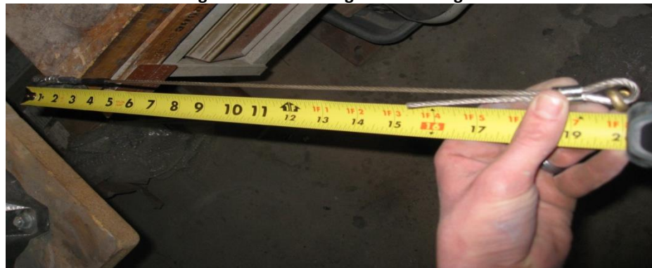
Figure 13 - Measuring Cable to Length
