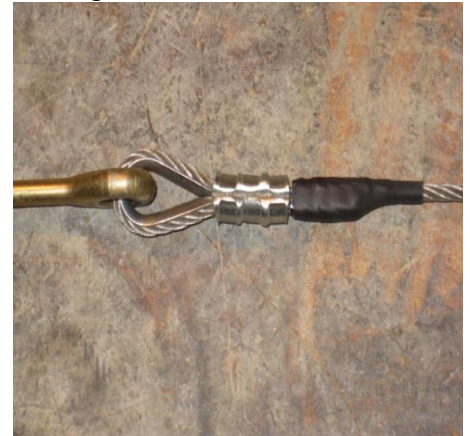
Figure 17 - Finished Cable End
