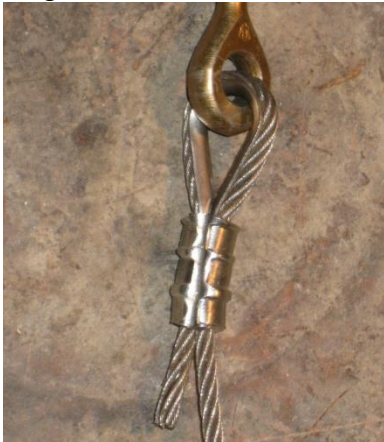
Figure 15 – Finished Cable End
