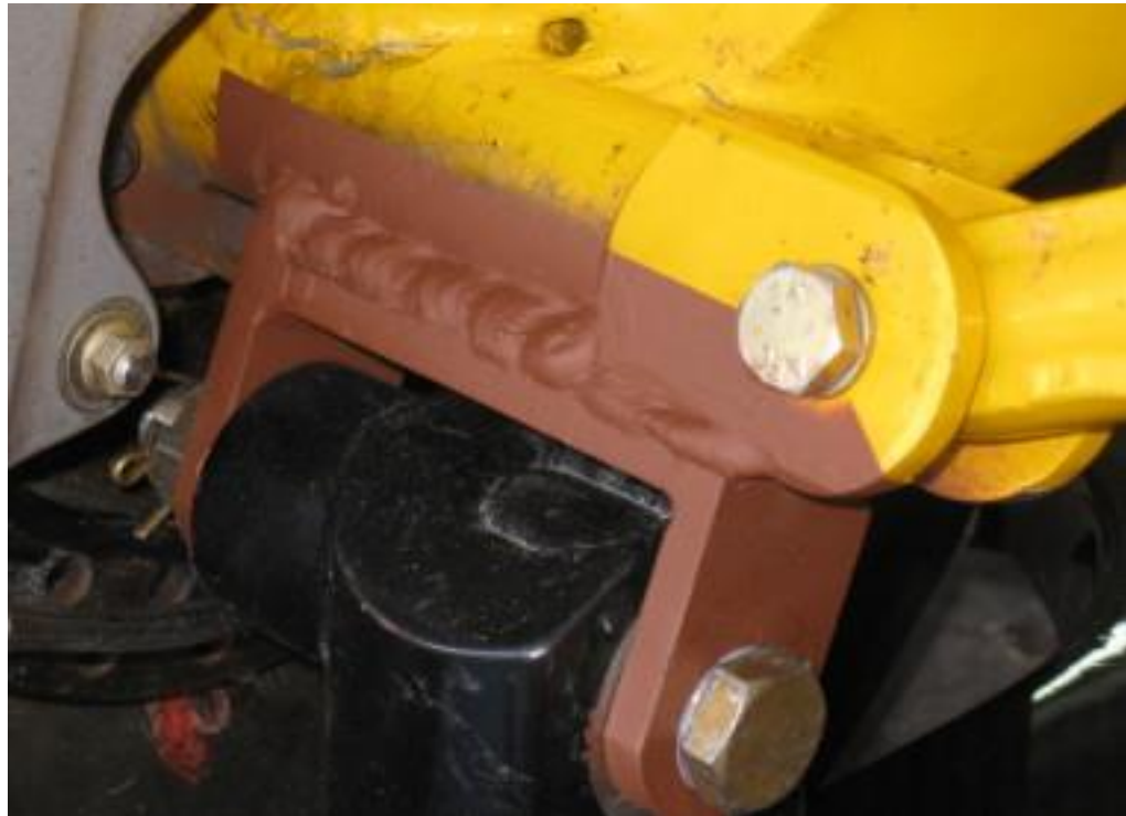
Figure 3 - Ski Attachment Bracket Weld
