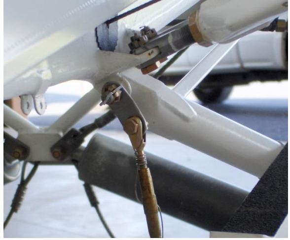
Figure 5 - Rear Two-Hole Tang Installation
