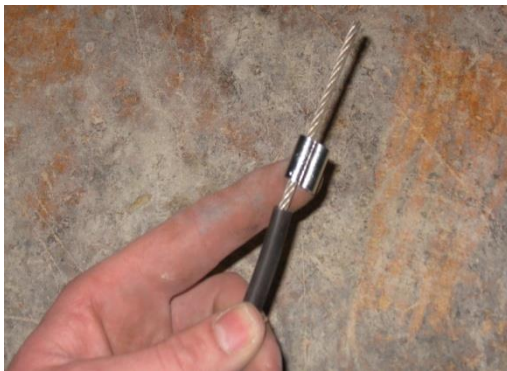
Figure 10 - Heat shrink & wire rope sleeve
