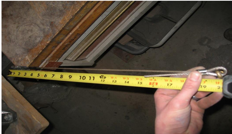
Figure 13 - Measuring Cable to Length
