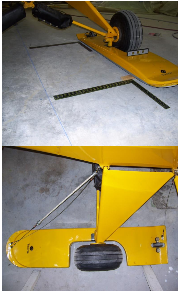
Figure 2 - Ski Alignment to Main Wheel
