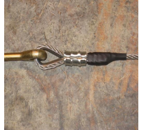
Figure 17 - Finished Cable End
