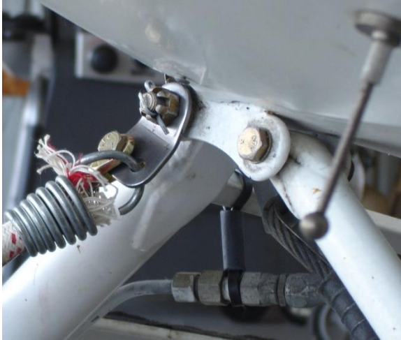
Figure 4 - Forward Three-Hole Tang Installation
