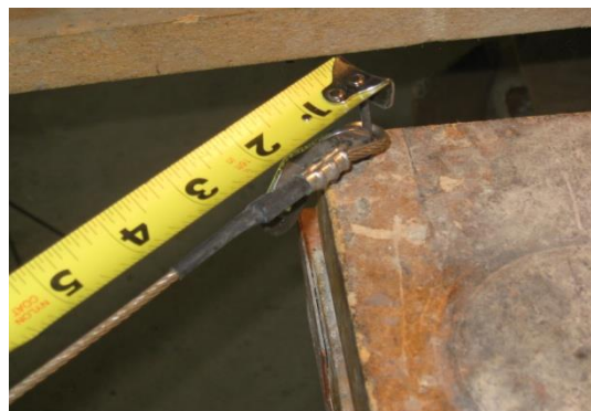
Figure 12 - Cable Measuring Fixture
