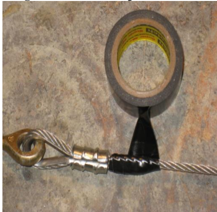
Figure 17 - Chafe Tape Installation
