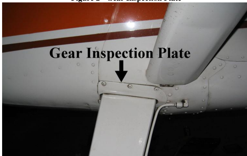
Figure 2 - Gear Inspection Plate
