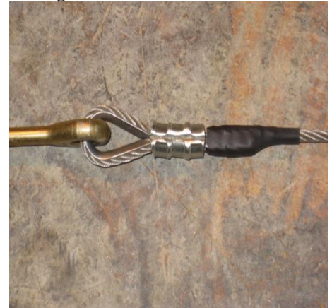
Figure 18 - Finished Cable End
