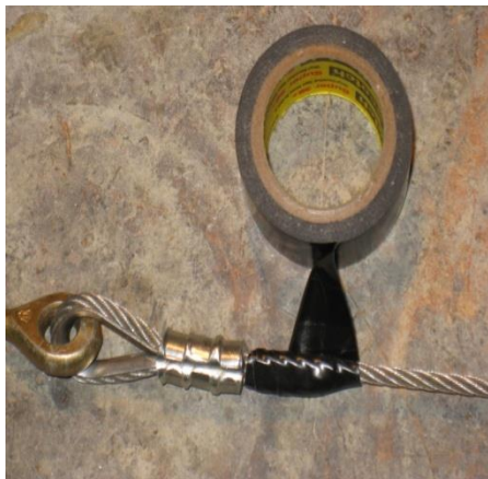
Figure 16 - Chafe Tape Installation
