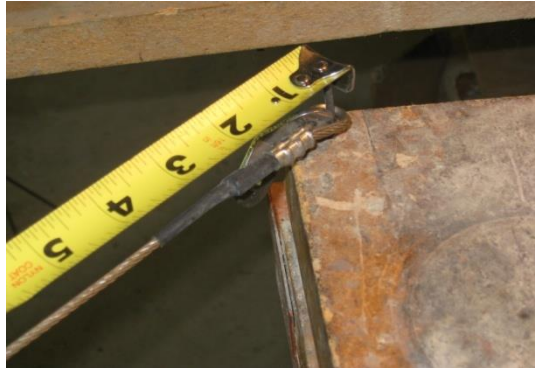
Figure 12 - Cable Measuring Fixture
