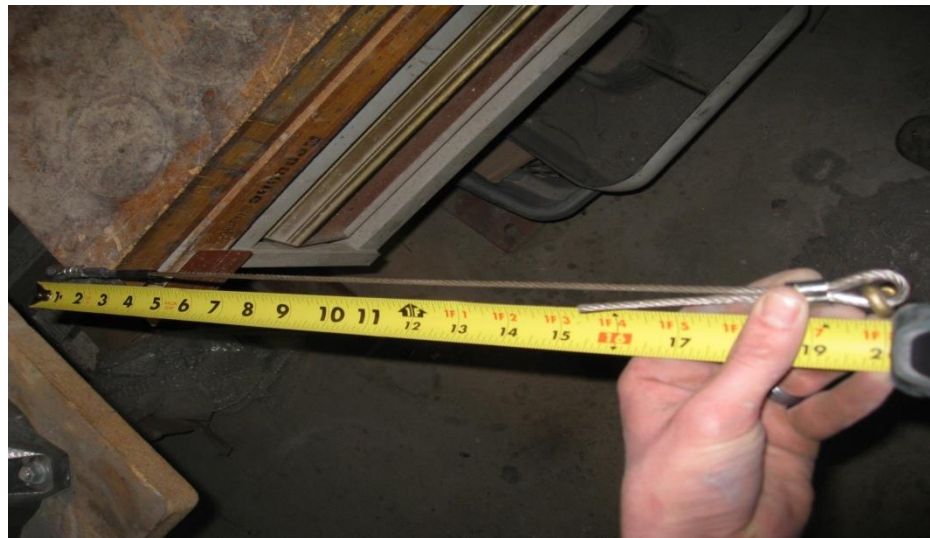
Figure 13 - Measuring Cable to Length
